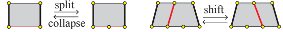
Figure 13: Split/collapse and shift are low-level operations on course and wale edges, respectively.
